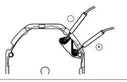
2. With the probes of the tester applied, place the solar cell unit at a distance of 5 cm under a fluorescent light of 15 to 20 watts, exposing the solar cell side to the light, and then measure the output voltage.
