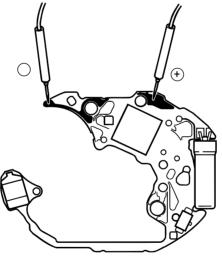
• Output voltage for the solar cell unit
