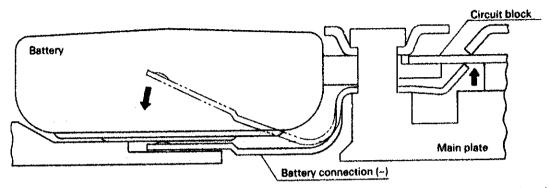
2) As the main plate is made from plastic resin, the conductivity cannot be obtained even when the (+) probe is attached to the winding stem. Be sure to connect the (+) probe to the battery connection (+).
