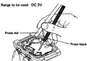
The pointer swings regularly: Normal The pointer does not swing regularly: Defective
