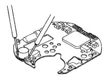
Result:  $40\Omega - 80\Omega$ : Normal Less than 400 — Defective More than 80Ω -
