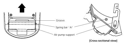
2) While squeezing the air pump with fingers, pull out the air chamber through the gap between the case hole and spring bar "A".
