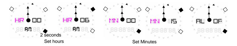
No action on buttons, for 3 seconds gets out ALARM ADJUST
