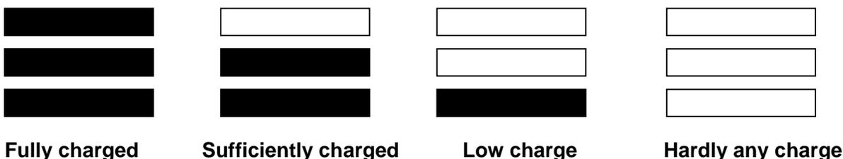
When none of the bars of the graphic display are lit, the secondary battery has essentially become completely discharged and the second hand begins two-second interval movement. Since the watch will stop due to insufficient charging if this state continues for about 1.5 days, sufficiently charge the watch by exposing to light.
