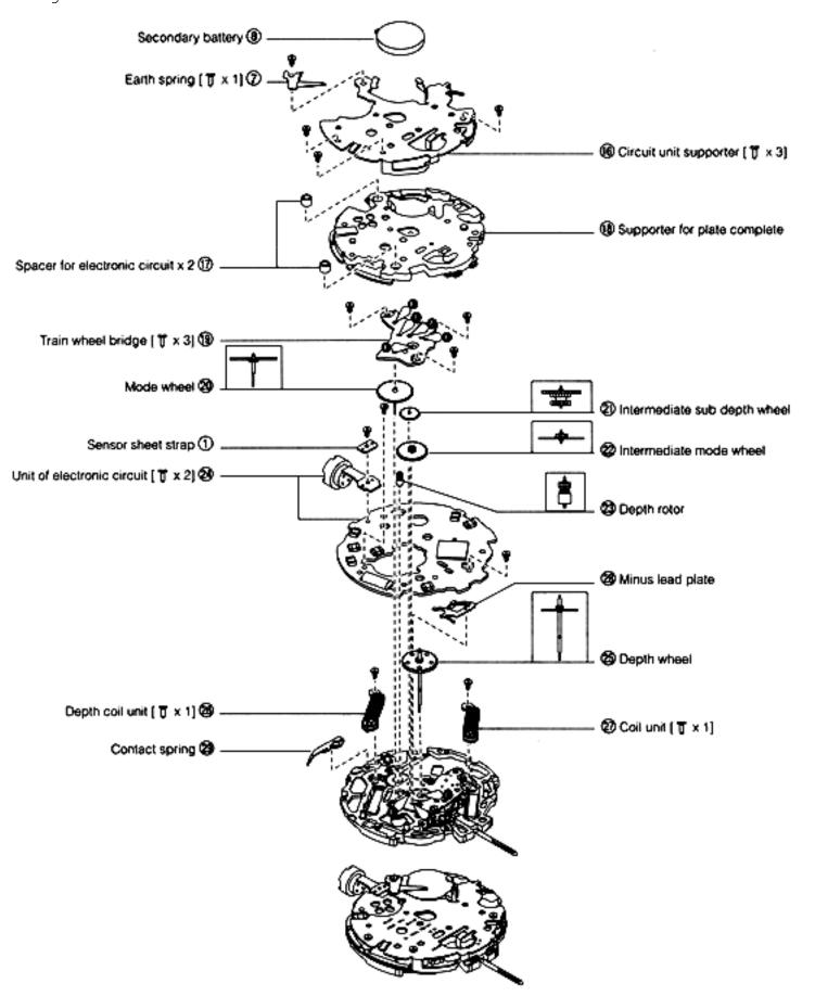
Use the movement holder No. B74 for disassembly and assembly.
