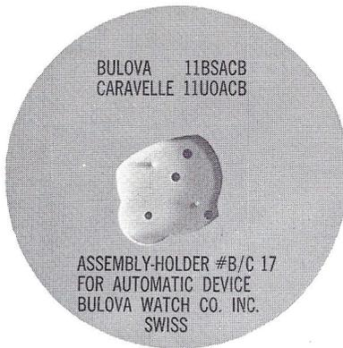
An alternate and much simpler method is to use the special BULOVA ASSEMBLY-HOLDER #B/C 17 for Automatic Device 11BSACB (Fig. 4) available at authorized BULOVA MATERIAL DISTRIBUTORS. When assembling merely follow the numerical sequence of Fig. 3 but hook the long ends of the springs #304 and #371 behind the stop pins in the HOLDER. When the assembly is complete, mount the entire unit onto the movement.
