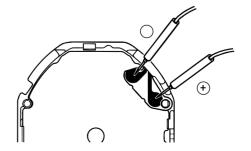
2. With the probes of the tester applied, place the solar cell unit at a distance of 5 cm under a fluorescent light of 15 to 20 watts, exposing the solar cell side to the light, and then measure the output voltage.
