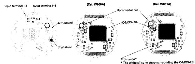
for Cal. W801A has a protrusion so that the circuit blocks for Cal. W801A and Cal. W800A can be identified.
