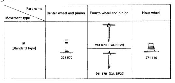
The types of hour wheel, fourth wheel and pinion, and center wheel and pinion are determined based on the design of cases.
