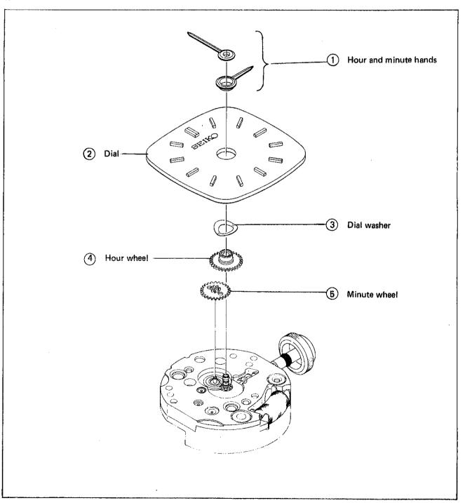
Disassembling procedures Figs.: ① → ②7
