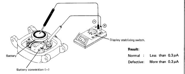
Set the display stabilizing switch of the tester to the "B" position.
