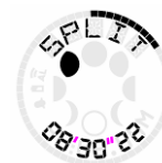
Display when chrono is frozen, pictograms blink because chrono is ON
