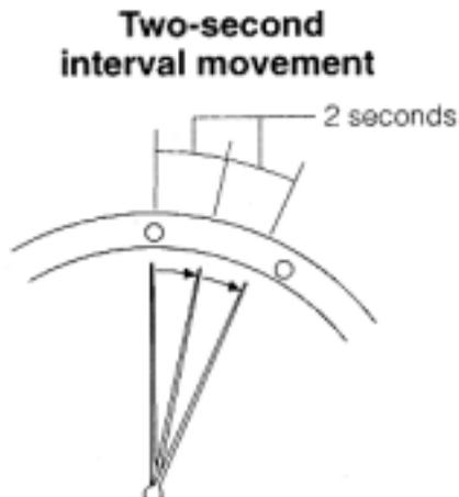
The second hand moves at two-second intervals to indicate that the watch is insufficiently charged. Although the watch will continue to operate normally at this time as well, it will stop after about 2 days have elapsed since the start of two-second-interval movement. Expose the watch to light to return the second hand to one-second interval movement.
