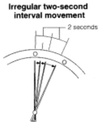
When the watch is again exposed to light after stopping, although the second hand begins to move, since the time is incorrect, the second hand moves irregularly at two-second intervals to indicate that the time is incorrect. Reset the time after the watch has been sufficiently charged. The second hand will continue to move irregularly at two-second intervals unless the time is reset.
