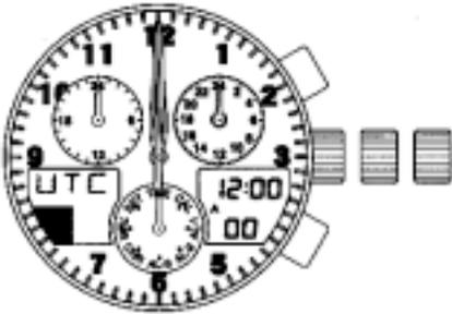
The watch stops when insufficient charging continues for about 1.5 days. When the watch is charged by exposing to light after having stopped due to insufficient charging, each hand is rapidly advanced to the base position and stops. Each hand remains stopped until the time is reset.
